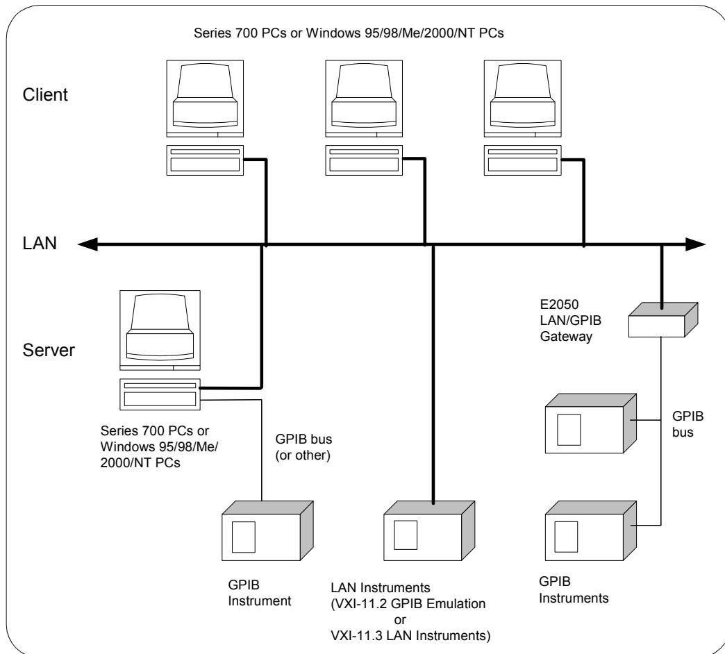
The LAN server is connected to the instrumentation or devices that must be controlled. Once the LAN server has completed the requested operation on the instrument or device, the LAN server sends a reply to the LAN client. This reply contains any requested data and status information that indicates whether the operation was successful.
